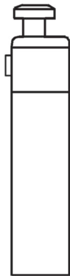
Radiator Detail Drawing Make from Balsa or Blue Foam and Nylon Window Screen
