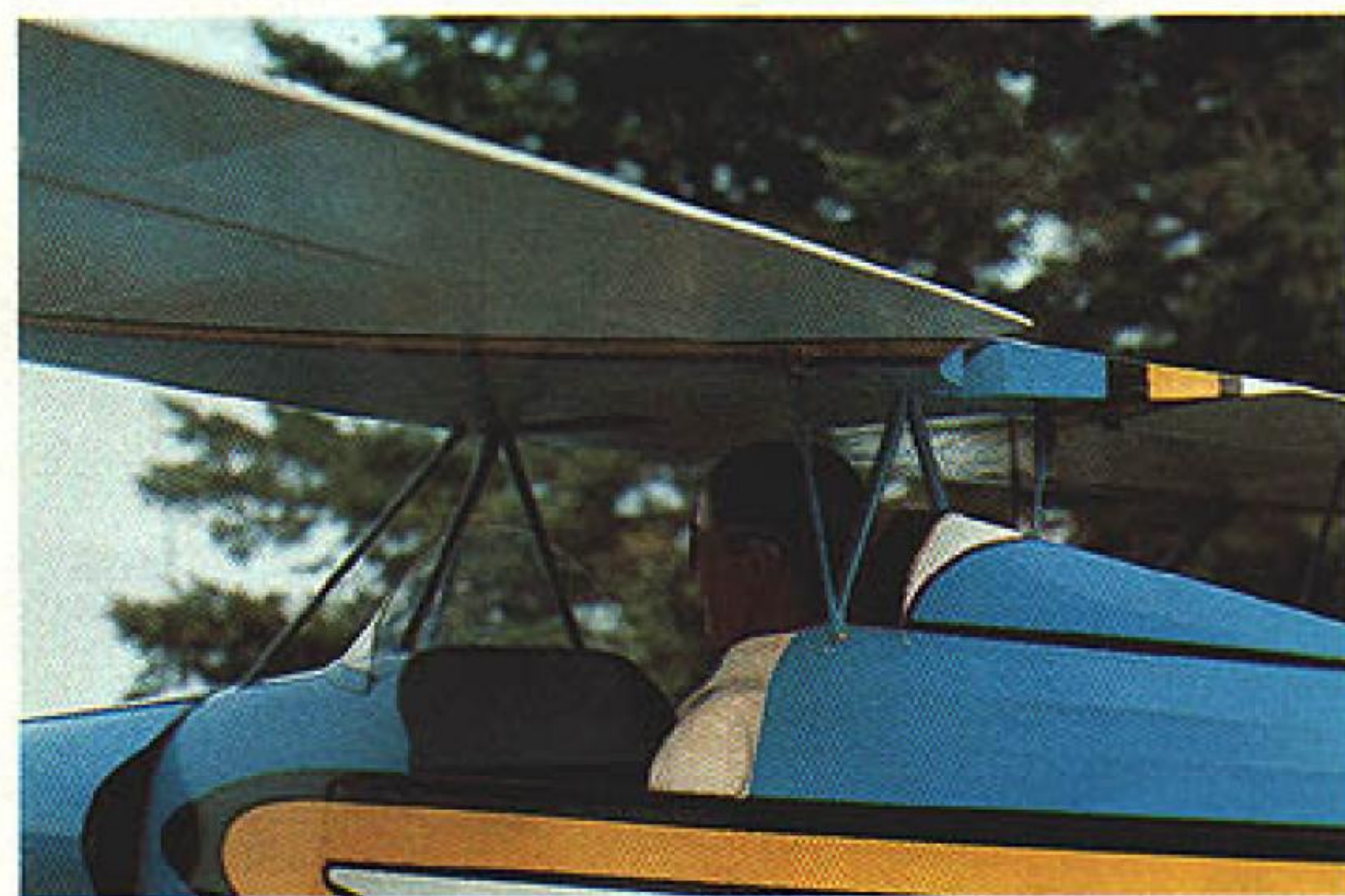
Steel wire cabane struts are anchored securely into fuselage, as they are the main load-carrying members. Note leather-covered headrest.
