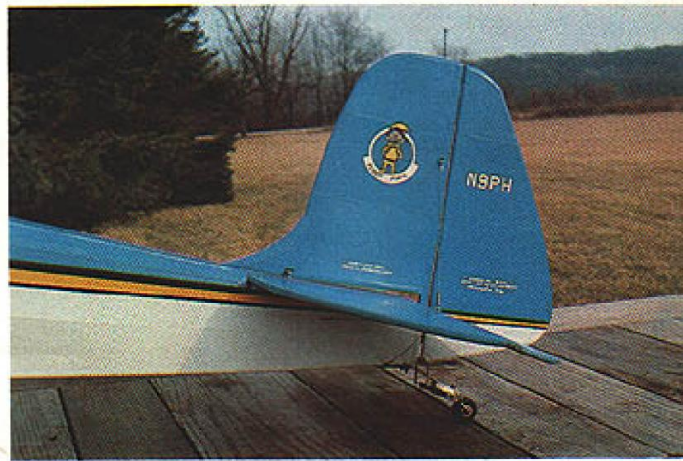
Tail surfaces are wire-braced on the model as on the original. Pixie logo was hand painted in oil colors on blank decal paper.
