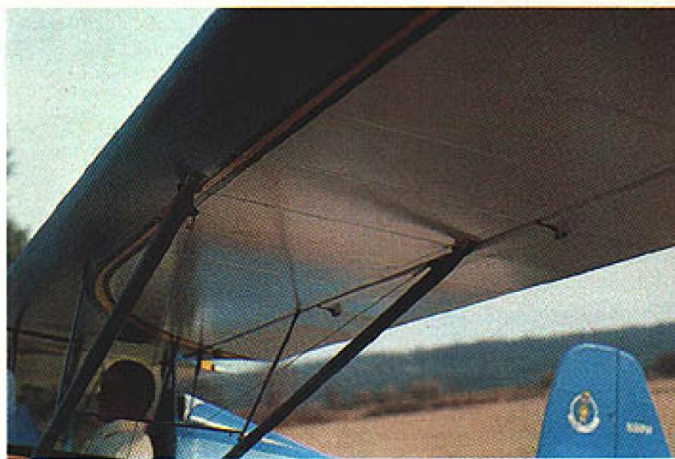
Wing struts on the model Pixie are a necessity because cabane struts are the pylon type. Jury struts are also functional.
