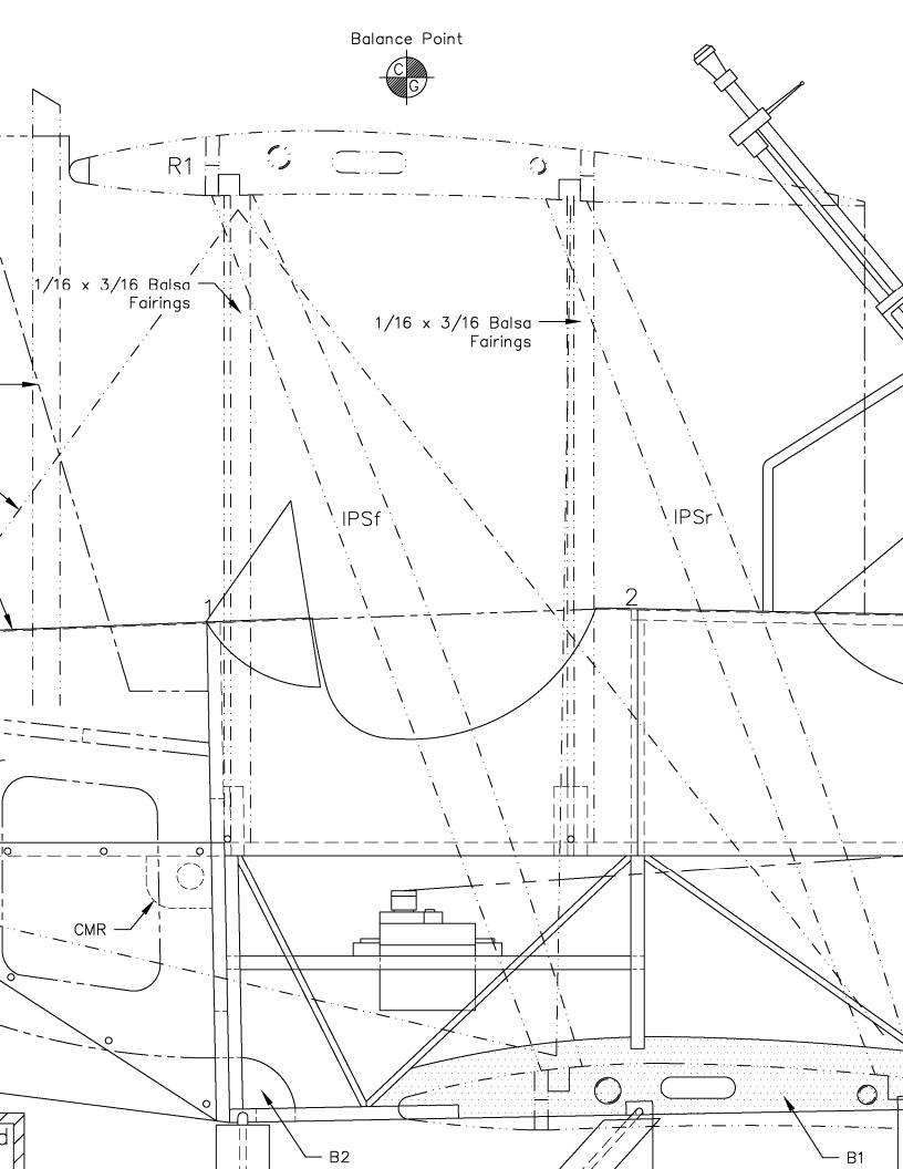
Note: The Dummy Engine is made up from .54" O. the Vac—Formed Plastic Cylinder Heads, 1/16 Alumin and 1/4" Triangle Stock. The Cylinder Assemblies glumm1 & MM2, flush with Former CF1
