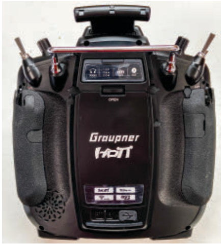
The back of the radio has battery access, a USB port along with an access panel for the headphones, and com, data, and DSC ports.
