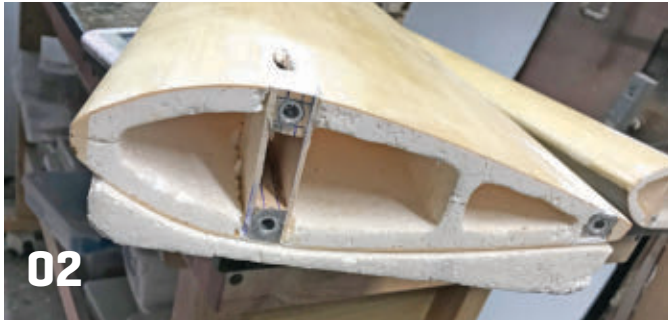
The wing take-apart hardware was encased in hard balsa then tied together with 1/8-inch vertical-grain balsa. It was then epoxied into the foam wing and sheeting.
