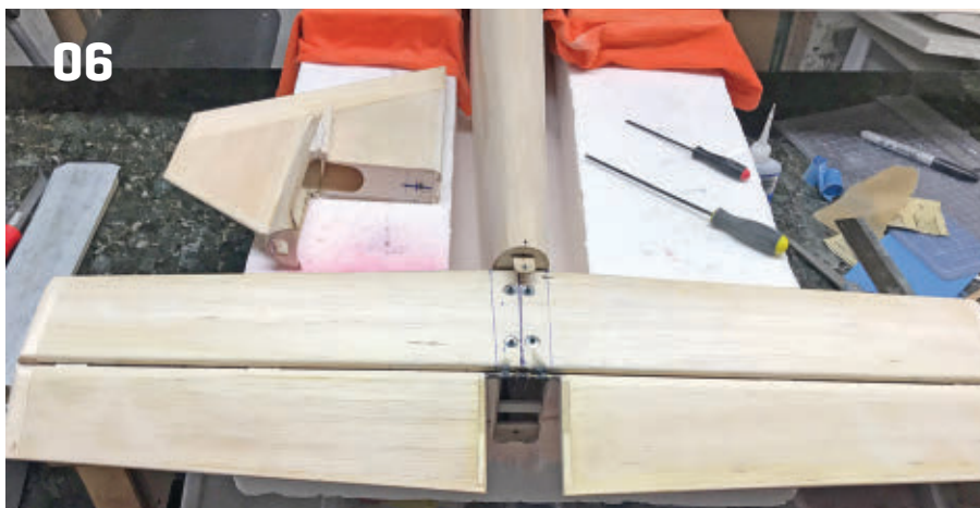
The stabilizer is bolted to the fuselage, rudder, and the back of the fuselage.
