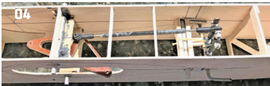
To hold the tube in place in the fuselage and as a bellcrank mount, 1/8-inch plywood was used.
