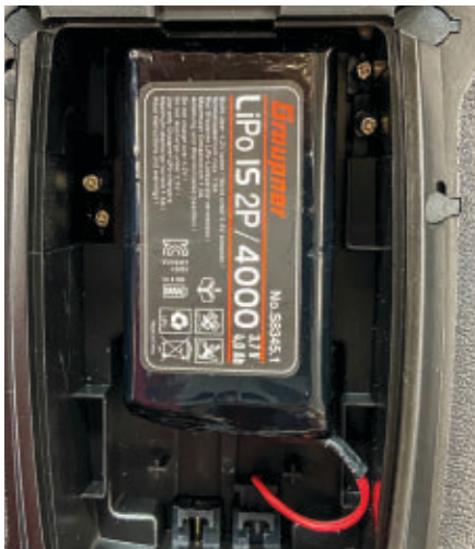
The battery is a single 4,000 mAh LiPo cell. A 9,000 mAh pack is an option.
