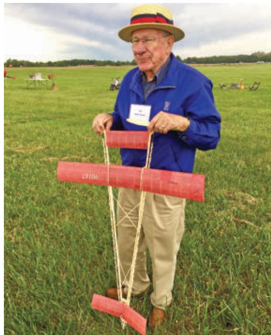
Grant Carson shows the simplicity of early twin-pusher construction. Despite flying backward (pointy end first), it produced a reliable and stable-flying model. Photo by Dorman Crawford.
