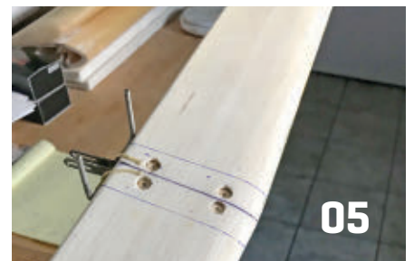
Shown are the four maple inserts in the stabilizer that the 2-56 bolts go through to hold the stabilizer to the fuselage.
