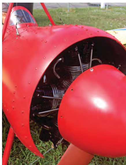
This view of the Morane-Saulnier Type N shows the five-cylinder UMS radial engine. Walt stated that the engine, available from CH Ignitions, is reliable and powerful.
