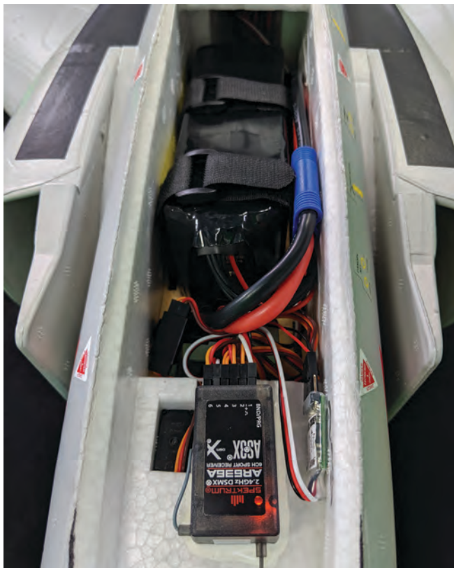
The battery bay is snug but can accommodate a wide range of batteries.
