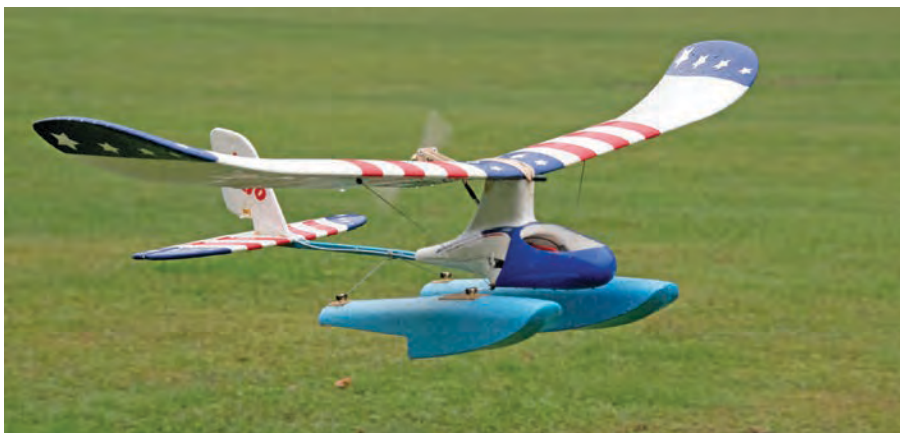
The author's Graupner Wingo, shown at the 20th anniversary NEAT Fair, now uses brushless power. Extended duration came with the much larger LiPo battery that was needed to maintain proper balance. Cardillo photo.
