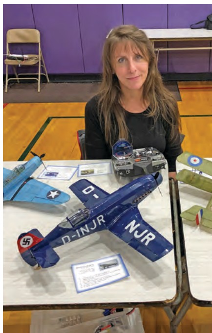
Sandy Cripps built this unique, 19-inch wingspan Messerschmitt Me 209 V1 prewar German racer. The model features handmade exhaust stacks, a vacuum-formed canopy, and a BL-180 motor.
