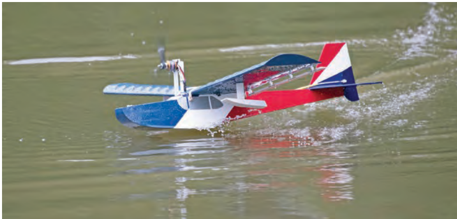
Terry Dunn's Puddle Master is enjoying its new life with brushless LiPo power and underlung ailerons. He refinished the floats, pylon, and forward fuselage as part of his successful restoration. Photo by Greg Cardillo.
