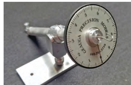
The torque meter is available with either a light (.012-inch) or heavy (.016-inch) wire element. Lindley photo.
