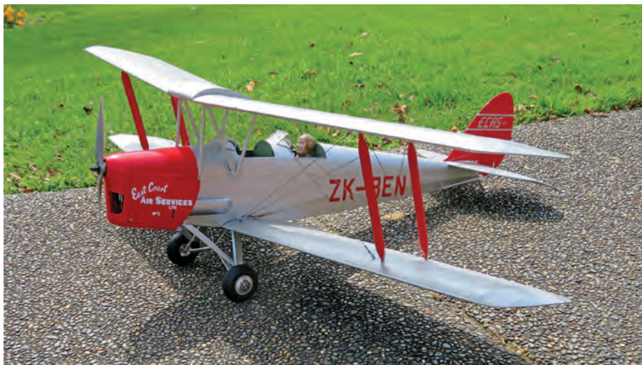
Another Hangar One kit is the classic de Havilland Tiger Moth with a 70-inch wingspan. It's built for .90-size engines. All of the kits have laser-cut parts.
