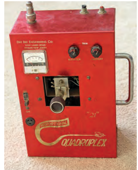
The Quadruplex 21, by Dee Bee Engineering, was the most reliable pulse-proportional system when it was introduced in 1964.
