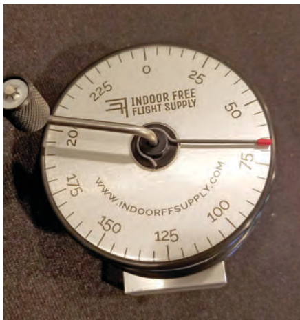
The winder face is marked in five-turn increments and includes a moving dial indicator. Photo by Dave Lindley.
