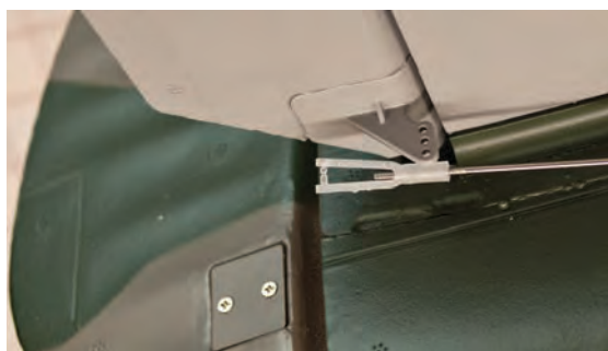
The elevator pushrod was too long and had to be shortened to work correctly.
