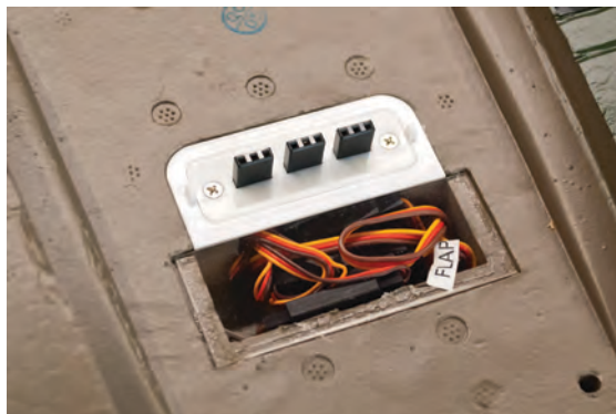
This built-in harness automatically connects the wing servos and retracts when the wing is mated to the fuselage.
