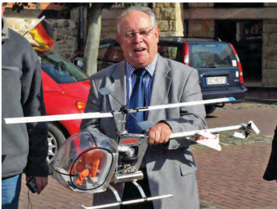
The fixed-pitch Schluter Heli-Baby was used by the author in 1976 to learn how to hover. Dieter Schluter, from Germany (shown above), is often credited with the invention of the RC helicopter.
