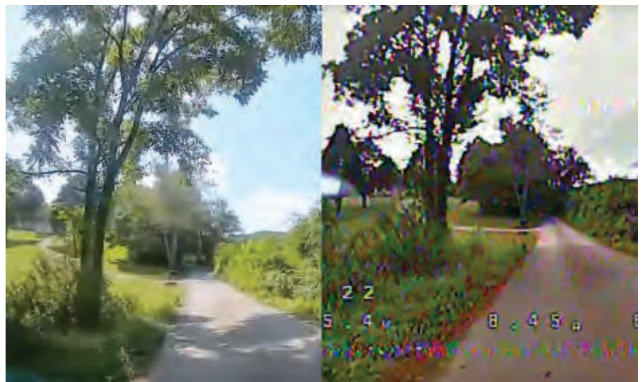
The DJI system's image, shown on the left, has a high resolution with "blockiness" as the image breaks up. The analog system's image on the right shows lower resolution with static.
