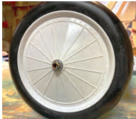
A WW I wheel was installed using a cotter pin and washer for a scalelike appearance.
