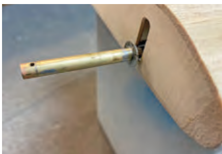
A brass axle bushing with a soldered washer stop was used for a WW I wheel installation.
