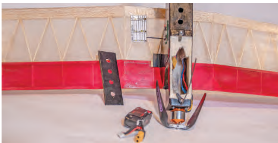
The battery for the electric-powered Lindy fits in the same space that carried lead ballast in the 1960 Lucky Lindy.
