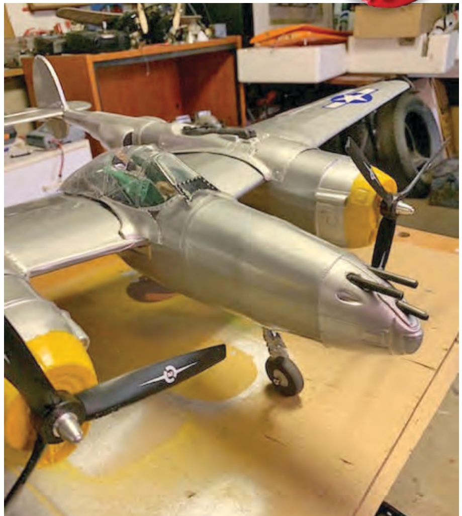
Michael Virr built his P-38 Lightning from the popular Guillow's kit. The electric RC modification included servo-actuated homemade retracts with mechanical down locks.
