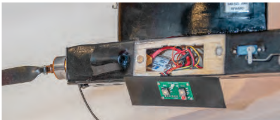
The original gas-powered Lindy had a built-up pylon that provided extra room for some of the electronic components.
