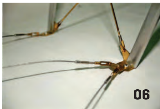
04. This photo shows what the cable end looks like after assembly and with the heat-shrink tubing applied.
