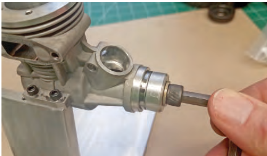
The ball bearing tool draws ball bearings in and out of the case without heat or damaging the bearings.
