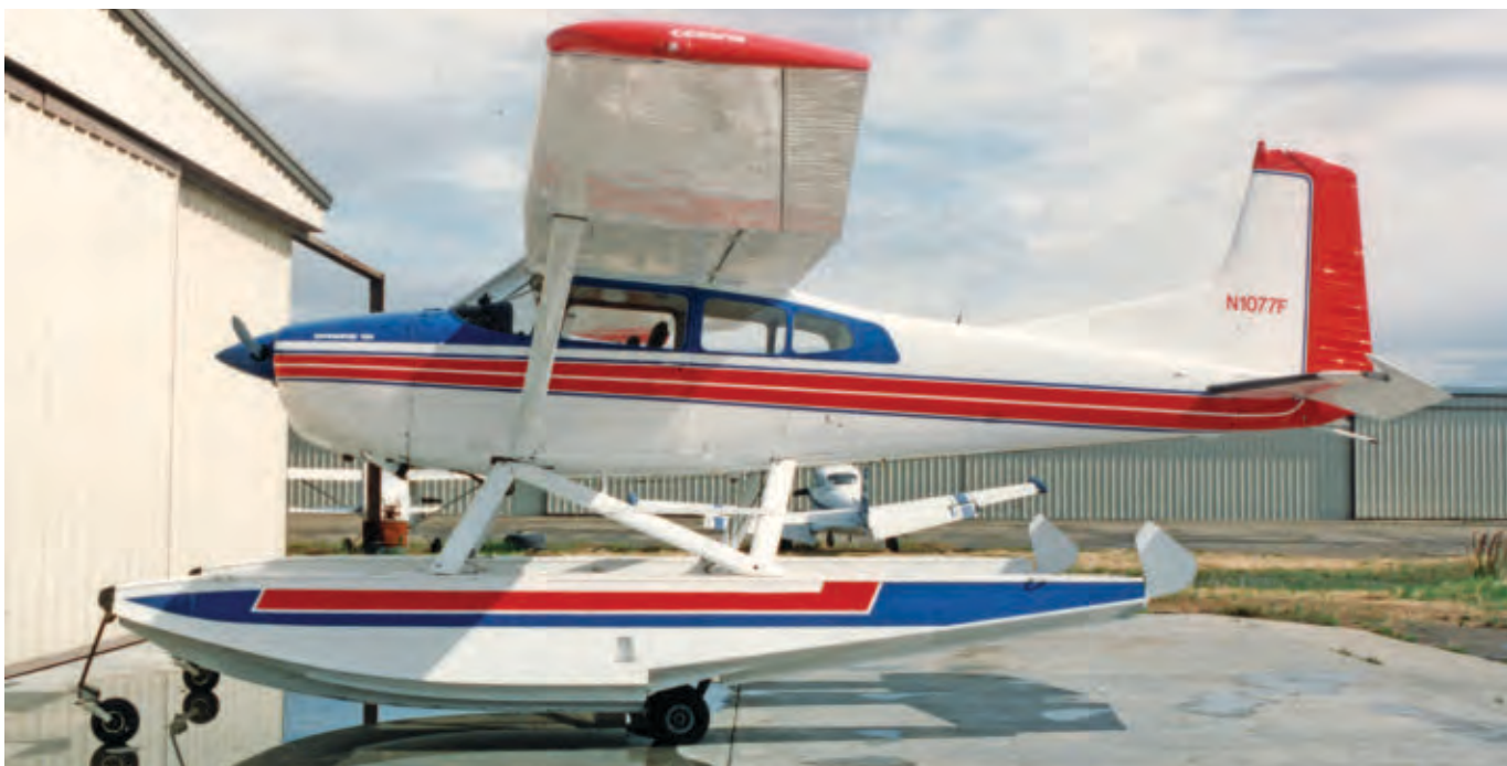
On this full-scale Cessna 185 Skywagon, the wheels are built into the floats. They retract, allowing the pilot to land on the water.
