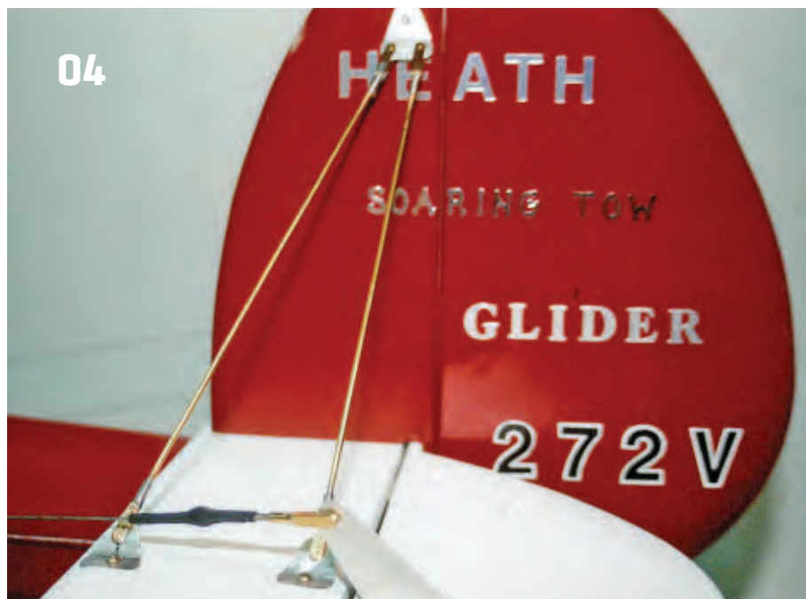
04. This photo shows what the cable end looks like after assembly and with the heat-shrink tubing applied.
