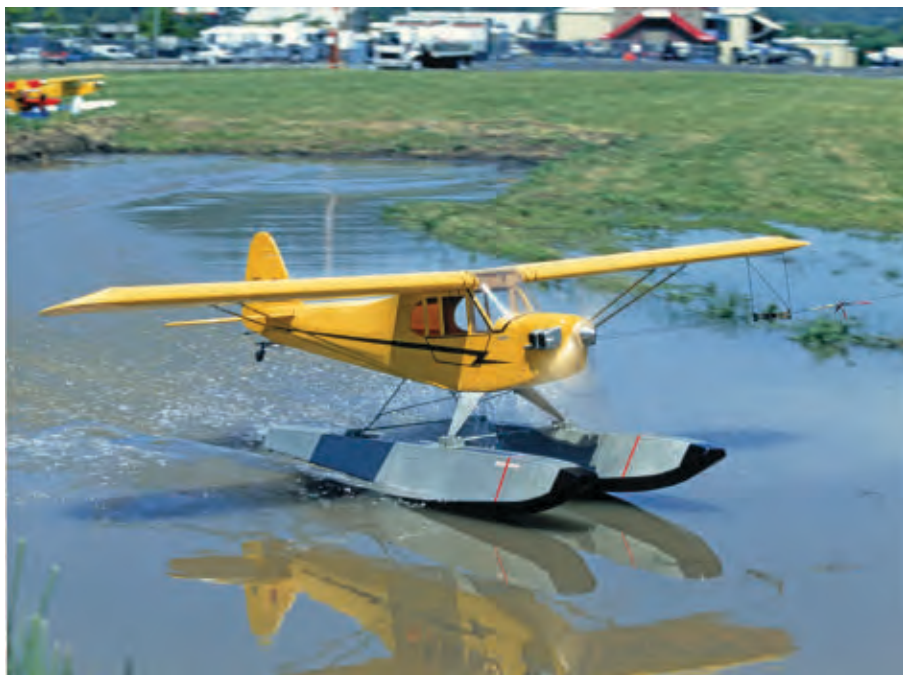
The author's 80-inch wingspan Piper Cub is shown on the step for takeoff at the 1998 Northwest CL Regionals float pond.
