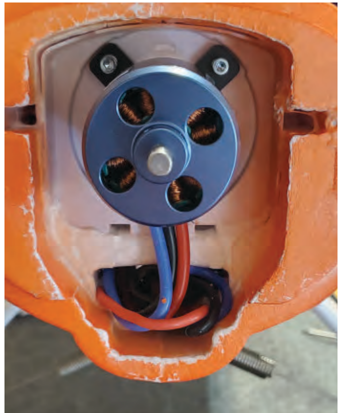
The Cub requires that the motor be bolted to the firewall and the motor wires be attached to the ESC. The process is easy; however, tucking the motor and ESC wire into the fuselage takes a little care because the ESC takes up a good portion of the available space.
