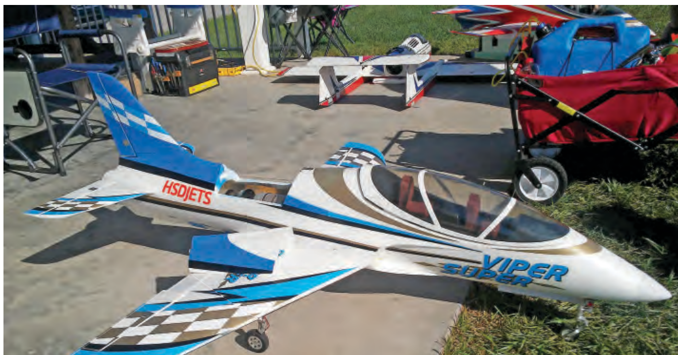
With the growing popularity of 45- to 60-newton turbines, smaller models, such as the HSD Viper that is shown, are filling pilots' needs for sport jets. This is a growing segment of the RC jet modeling community.
