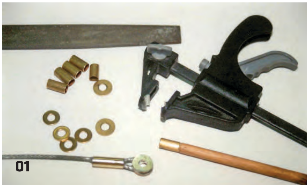
01. A fine file is used to clean up the soldered cable ends. A clamp is modified (notice the jaws) to hold the cable during assembly. A completed cable end is shown, along with brass washers and tubing.
