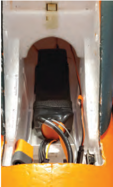
A multiposition, quick-release battery tray makes battery swaps easy. Nonslip shelf liner was put at the bottom of the tray, which stopped the battery from shifting.
