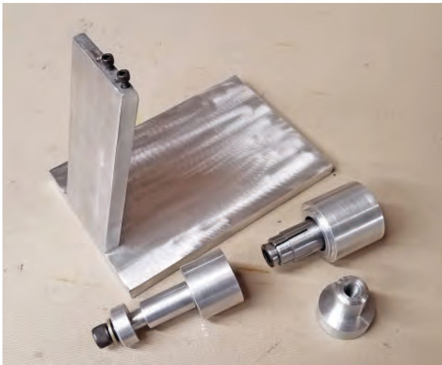
This Triple J Fabrications Nelson/Jett ball bearing tool and engine stand are handy for working on Q-40 Pylon racer engines.
