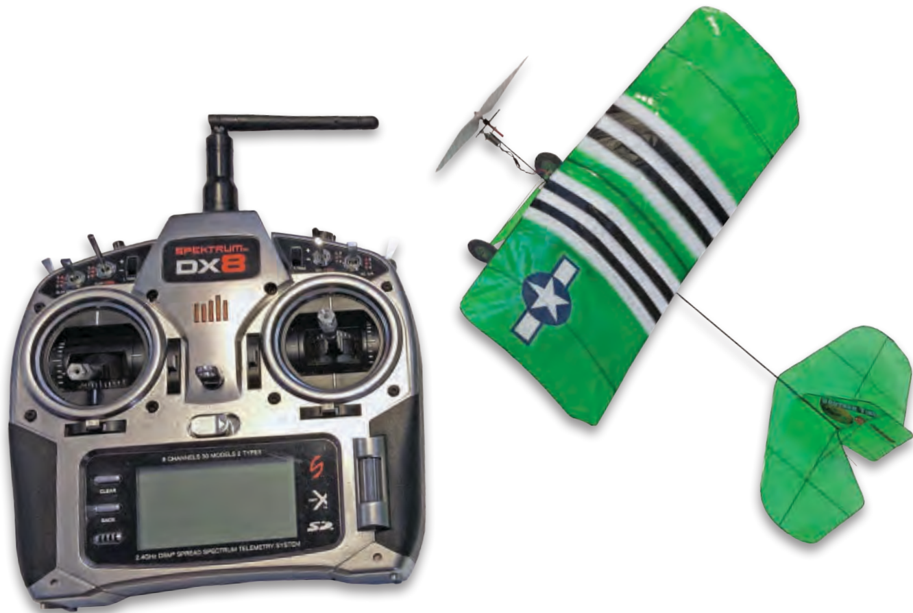
The small size of the 9-inch wingspan, two-channel model is apparent next to the author's Spektrum DX8 transmitter.
