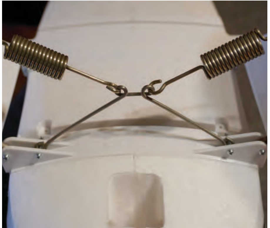
A combination of articulated, shock-absorbing landing gear with large tundra tires ensures that the Cub can stand up to imperfect landings or less-than-ideal flying sites.
