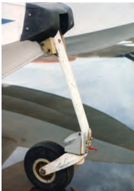
This is a typical nose wheel on a full-scale float. The gear swings up then retracts back into the float if the pilot wants to land on water.
