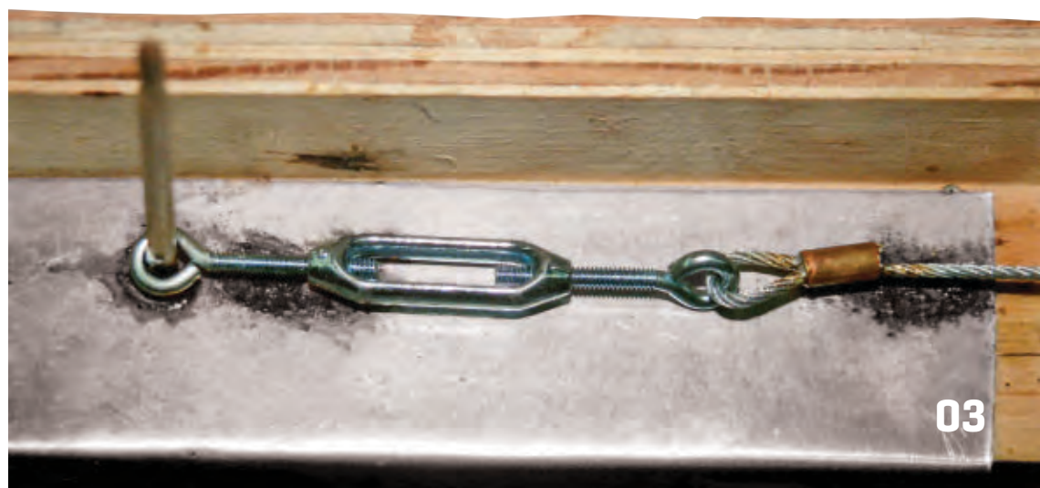
03. This shows a 2-inch piece of wood across the workbench with aluminum sheet stock placed under the work area. A large-scale cable end has just been completed.
