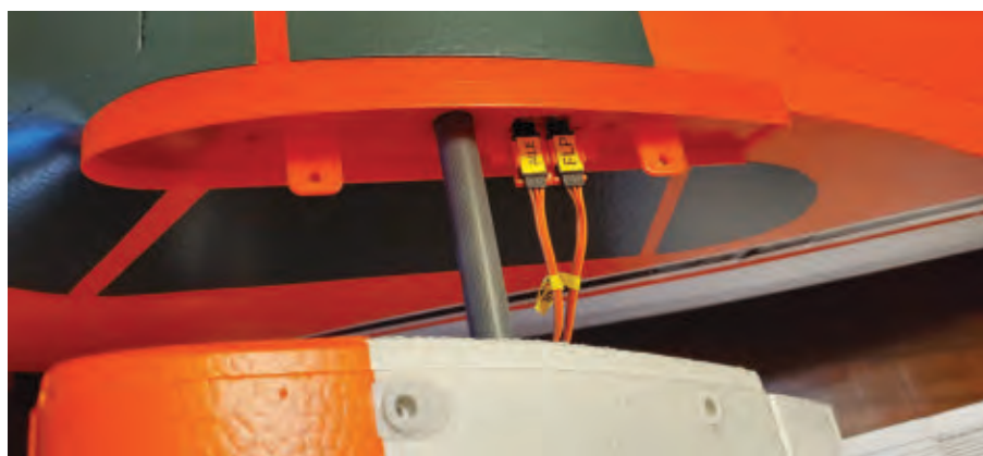
The wing halves slide over a carbon-fiber wing tube and the aileron and flap servo leads must be connected. The female ends of the plugs are captured in the fuselage, but you still need to plug them in.
