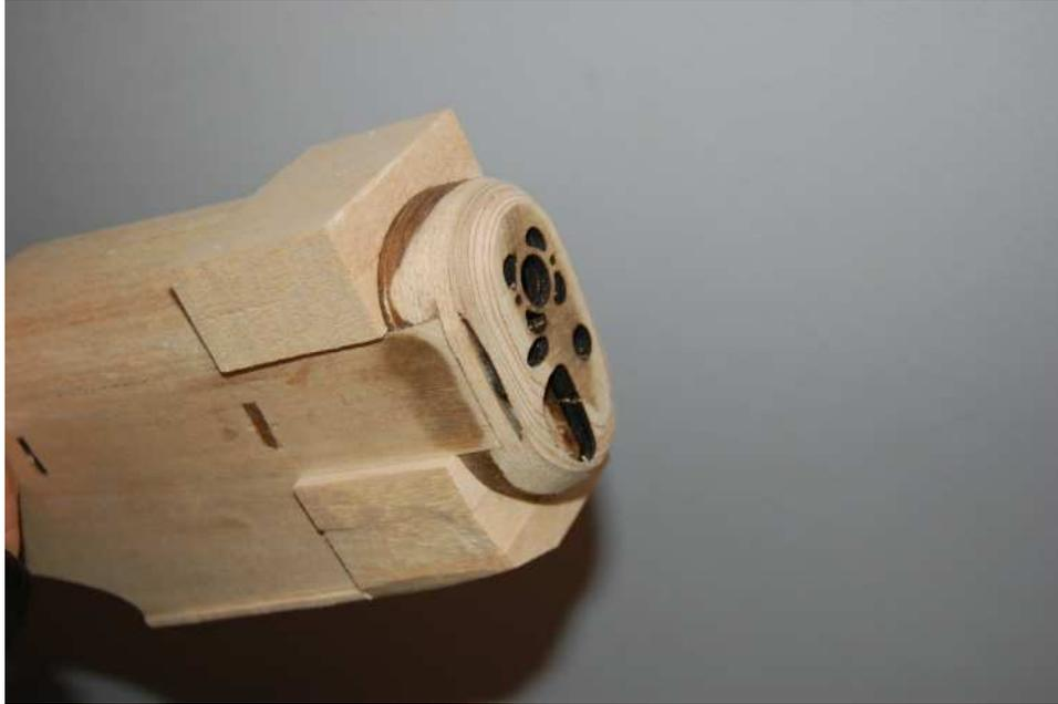
The blocks for the upper hatch and lower cowl are not included in the short kit. I used half inch balsa to glue them up. Use Epoxy on the lower block for strength
