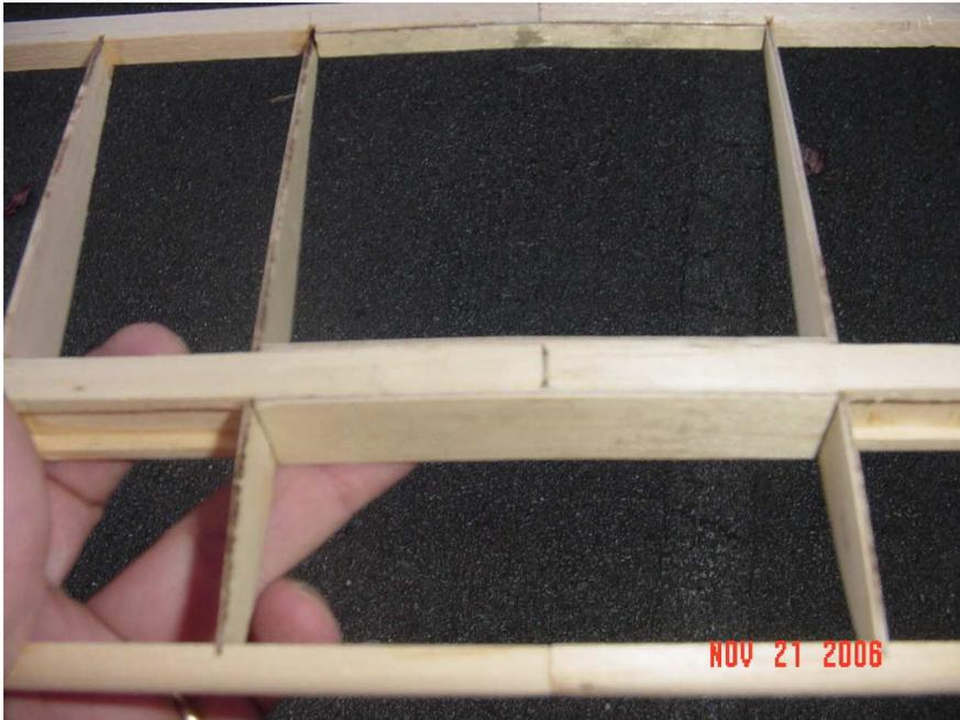
Plywood wing spar doublers are added then the wing center ribs were added. This is not the normal way things are done but it worked for me.
