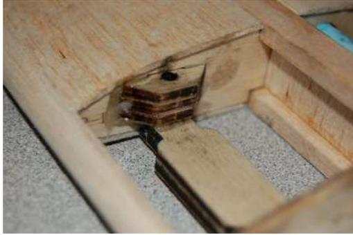
3. Glue the landing gear blocks to the L-3 stack and ribs, using epoxy.
