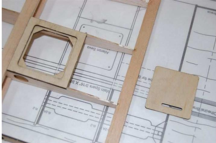
10. Install aileron servo mounting plates.
