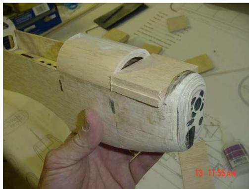
16. Using razor plane and sanding blocks, shape the nose blocks along with the bottom and top hatch blocks. (To expedite the process a power disc and belt sander was used to rough sand the prototype to a rough shape)
