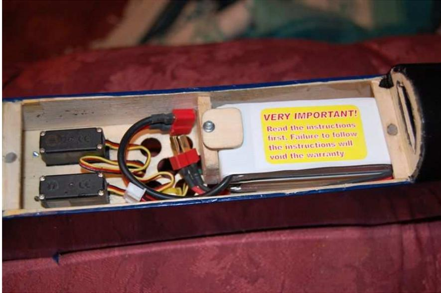
Do not depend on the hatch magnets to be enough to hold the battery in place while flying (Ask me how I know) I use the forward magnet mount to anchor the end of the battery and a swing around plywood plate to hold mine in place.
