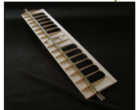
Center section showing all lower surface sheeting, dihedral braces, balsa/carbon spar with Kevlar tow and mounting blocks.
