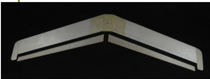
Complete canard structure ready to cover showing tip blocks and fiberglass reinforcement at dihedral breaks.
