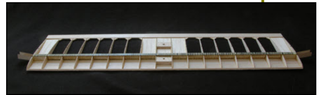
Center section structure without upper surface sheeting.
