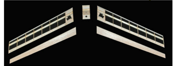
All five canard structures (two servo method) without any upper surface sheeting.
