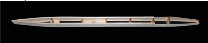
Basic fuselage structure showing sides, all formers, tail stock and ply mounting plate for tow hook.
