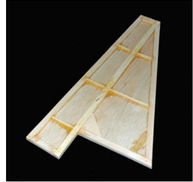
Vertical stabilizer internal structure before addition of right side sheeting.
