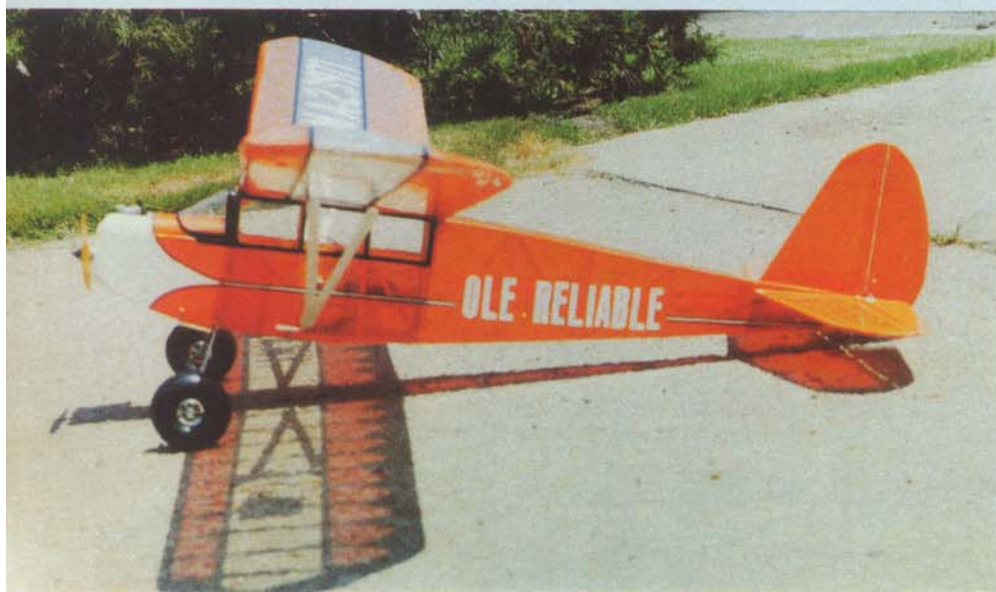
What you see when you stand ready, transmitter in hand, for that first flight. If you balanced the model properly, and checked for warps, a successful R.O.G. is practically guaranteed.
