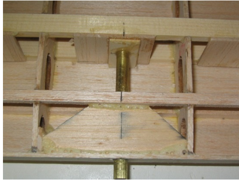
30 Pitot Tube Mount in Wing
