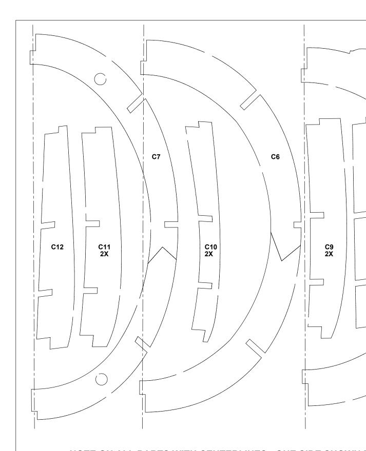
NOTE ON ALL PARTS WITH CENTERLINES: ONE SIDE SHOWN I MAKE A LEFT AND RIGHT SIDE FOR EACH OF THESE PARTS
