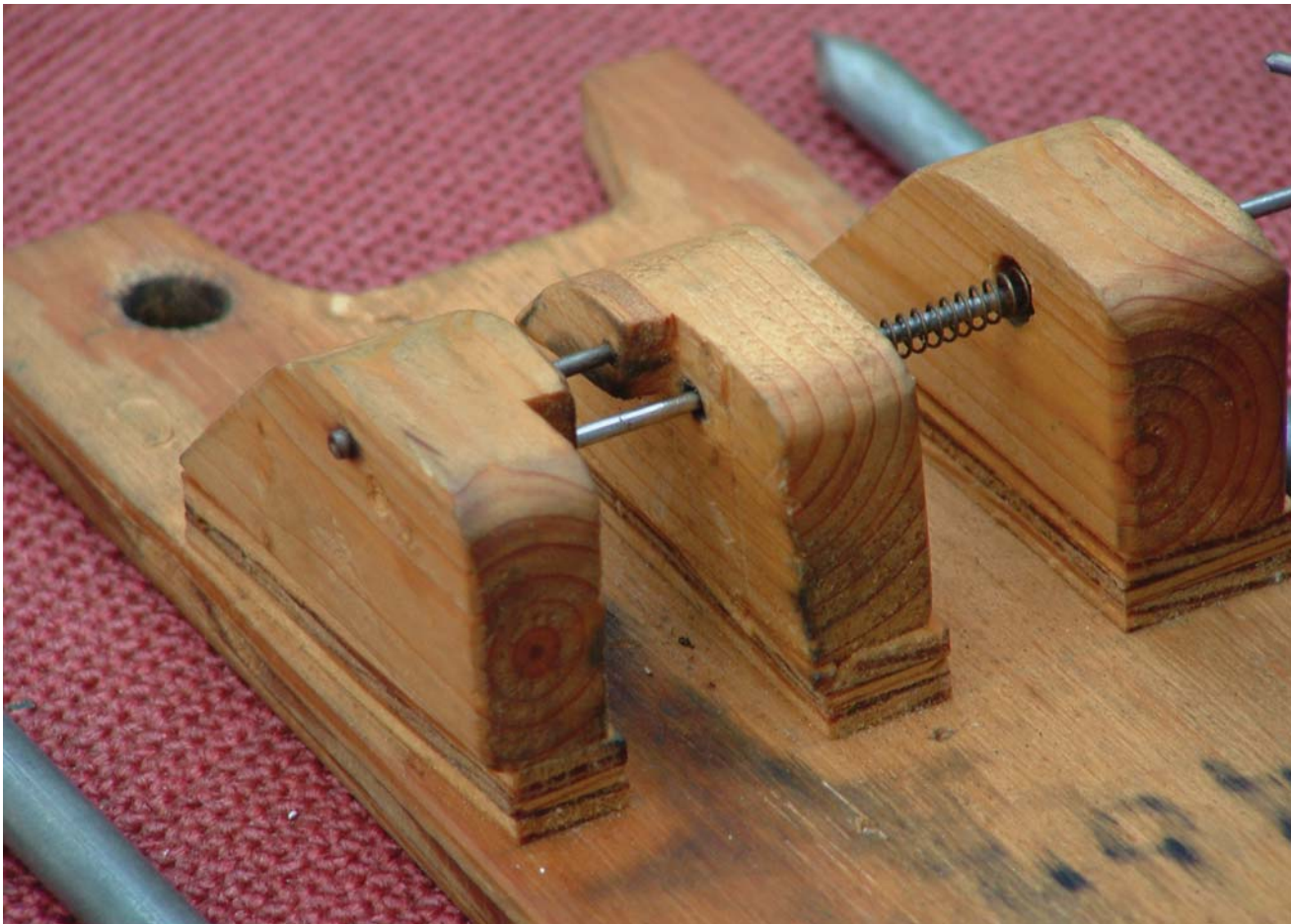
This close-up of the prototype Stooage, shows the simple spring loaded release, typical of most stooages. A trip line to the center of the circle gives the pilot full control of the launch.
