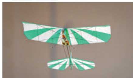
Gordon Johnson flew his 13-inch, curved carbon-fiber Stik Citabria. The model's wing is built with 12% camber. Sawn photo.
