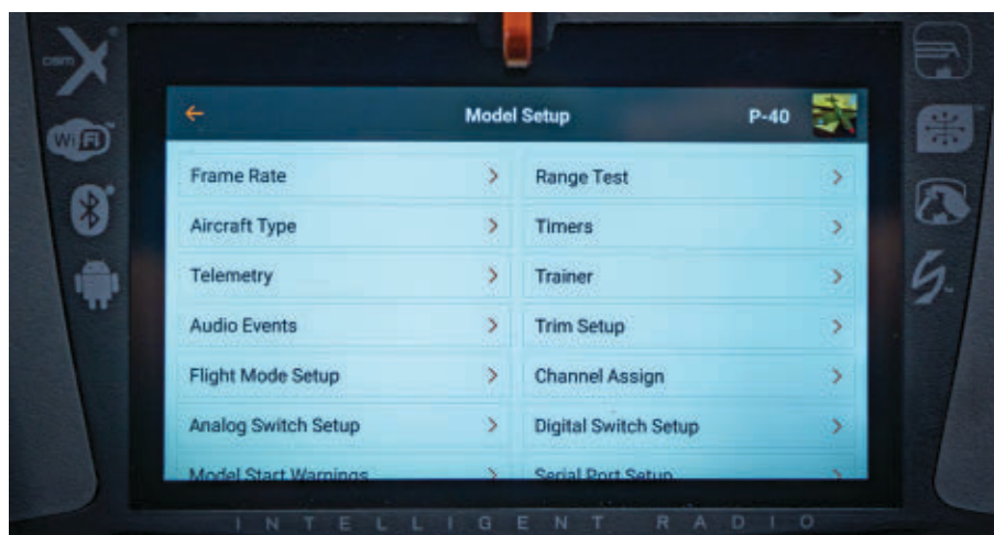
The Model Setup menu features are used for basic aircraft setup configuration. The menu list varies by model type.
