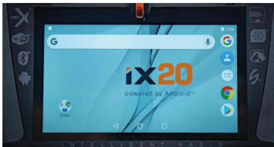
The Android Home Screen contains all of the applications that are loaded in the iX20. Shortcuts to applications can be moved onto the home screen for easy access.
