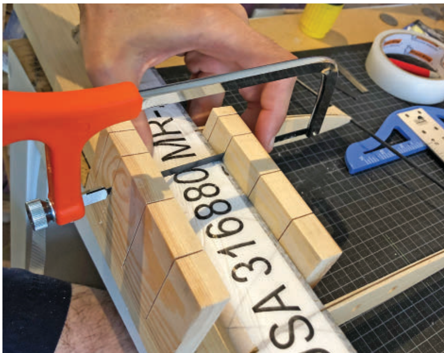
A saw guide, such as the one shown, can be helpful for making precise cuts when splicing wing parts together.
