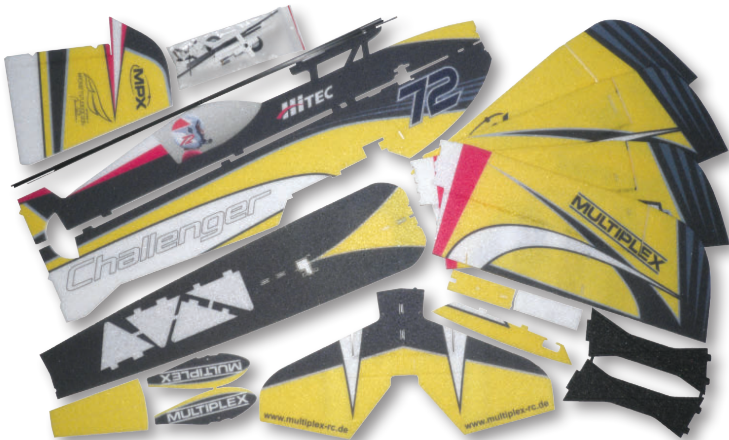
This is how the flat EPP foam, with its colorful preprinted scheme, comes out of the box.
