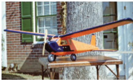
The author's original Royal Rudderbug was built from a Berkeley kit in 1953. It was flown with a Webra .15 cubic-inch diesel engine without a throttle and controlled with a simple escapement.
