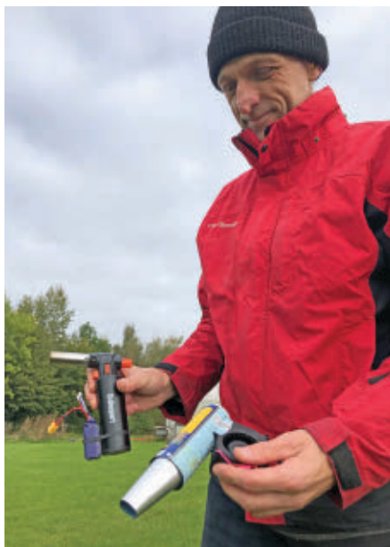
Ole Bjerager is shown with his heat gun at the Penguin Club outside of Copenhagen, Denmark. The small butane torch provides the heat, and a CPU fan driven by a small LiPo battery provides the airflow. The aluminum cone channels the air and provides a shield from the direct flame.
