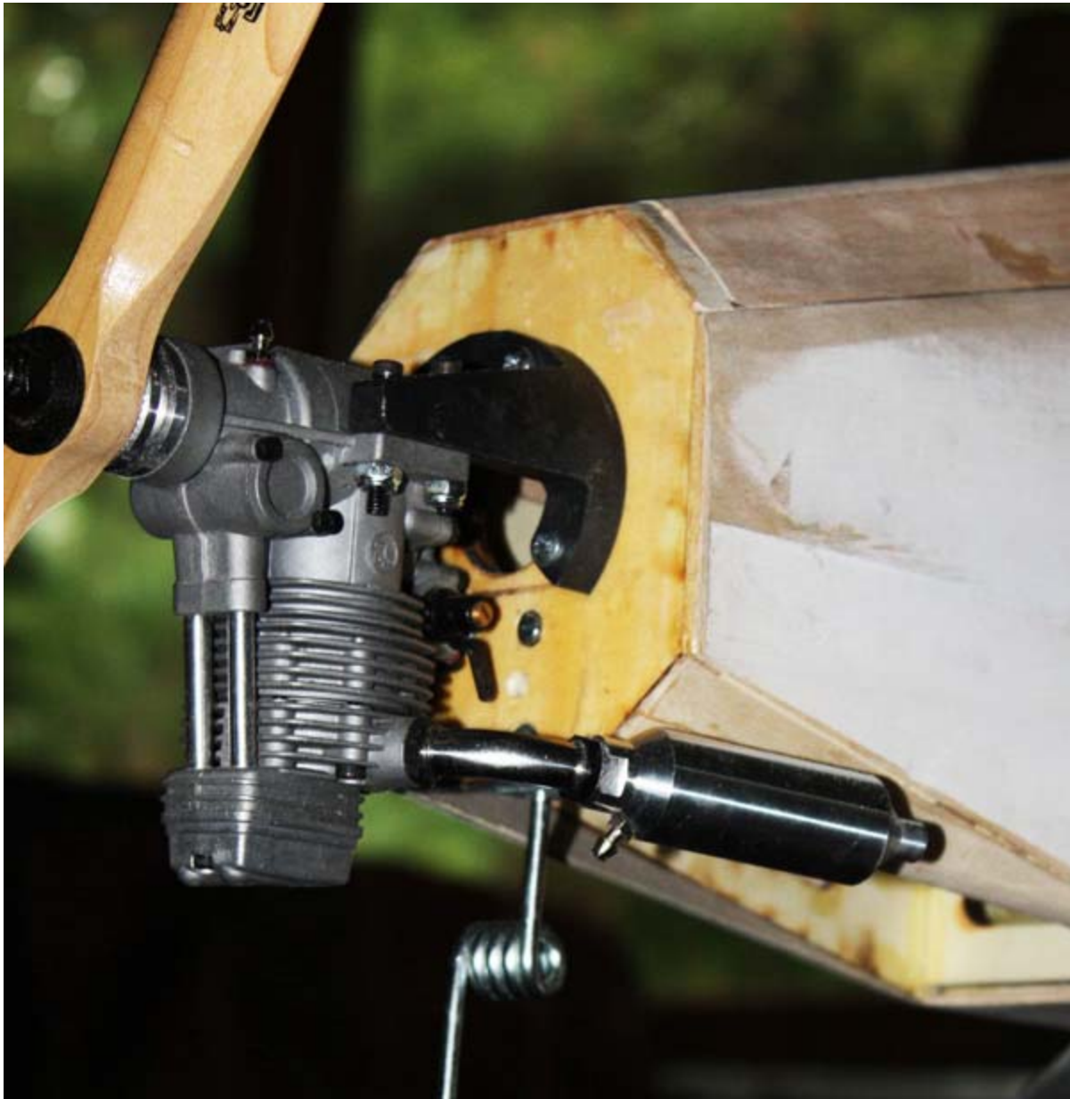
The engine in my model is a Magnum .52 four-stroke, which is mounted inverted.
