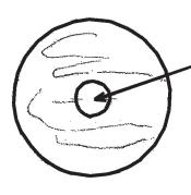
Clearance hole for rear of motor
